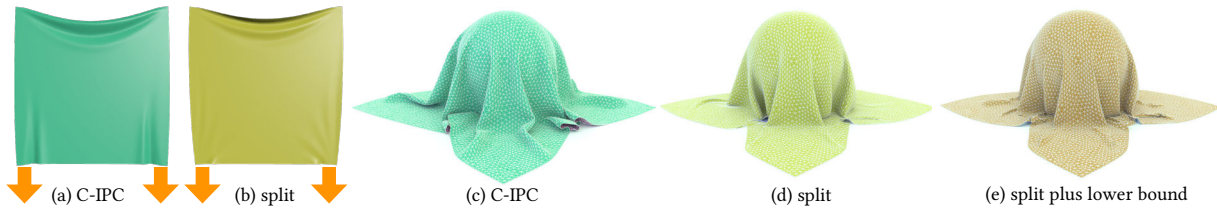
Fig. 14. Comparison of C-IPC’s fully coupled strain limiting model with standard splitting models highlights the differences between the fully coupled solutions in (a) and (c) and the artifacts generated by splitting strain-limiting solves from elastodynamics in (b), (d) and (e). Here we see that with splitting resulting large errors in elasticity (membrane and bending) can generate incorrect wrinkling directions (b), severe compression artifacts (d), or even numerical softening as in (d) and (e).
